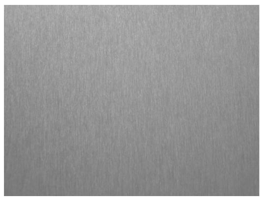
Lindner aluminium ceilings can be ordered with INOXlook appearance on request. The surface 'INOXlook' is created by special rolling and anodizing processes and is similar to a grinded stainless steel surface (grain 180).
